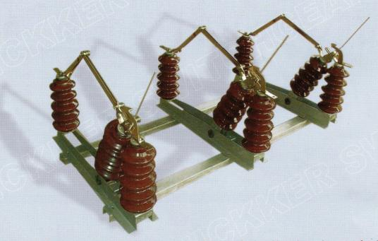
The outdoor interruptor switches contained in this list are designed for load breaking duties on feeder lines and ring main circuits or transformer circuits (in conjunction with HRC fuses or cut out fuses). They cover the rated voltage of 12/17, 5 kV up to 36 kV at rated currents of 200, 400 and 630 A. Different types are available the details of which will be provided on request.
